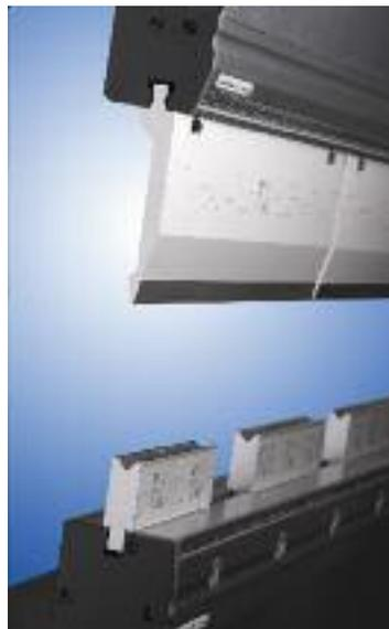
chined with self-seating grooves for use with Wila American Style hydraulic clamping systems, for quick setups.
